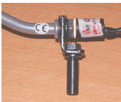
Ensure the Lunima 6 arm is secured firmly to the pole fitting
